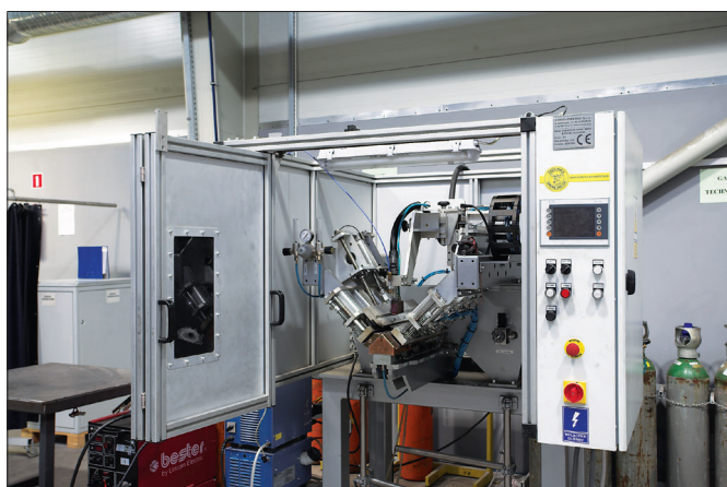
Automatic welder for SWN cabinets bodies
