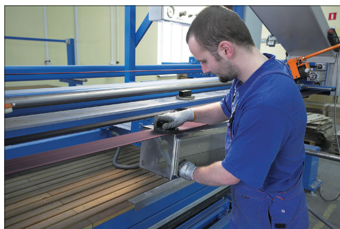
Welds machining for stainless steel cabinet body
